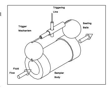
dock until the mark you've made is touching the water. If the sampler tends to float instead of sink, drop the sampler from a small height into the water. The white balls must flood if the sampler is to sink. To capture the sample, take a firm grip on the line then pull **sharply** upward. A **quick** tug of only a few inches is preferable. Slowly pull the sampler back out of the water.
