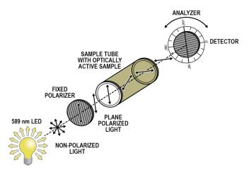
Figure 1: Schematic of the Polarimeter
