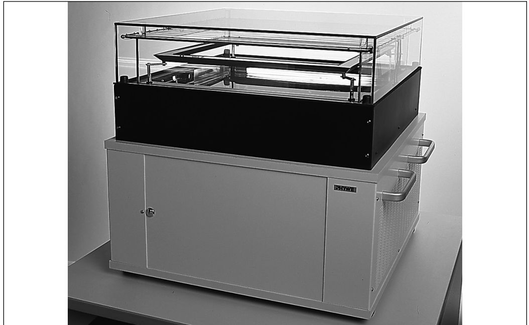
Fig. 1: Diffusion cloud chamber PJ45, 09046.93.
